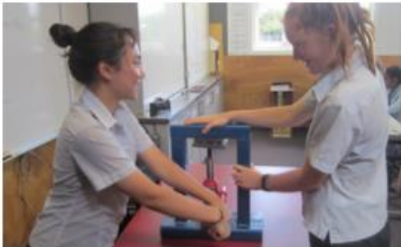
Yena and Sophie press forming copper sheet to make a dome
